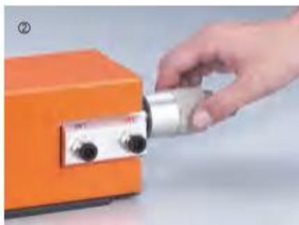
② 根据所需压接的端子直径来调节压接口的大小。(正方向旋转为加大口径，反方向旋转为减小口径) Adjust the size of nozzle according to the diameter of the clamped cable end-sleeves you required.(Increase caliber by twisting clockwise
