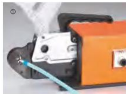
① 先把管形端子和相配电源线装好。 Assemble the cable end-sleeves and the power supply cord at first.
