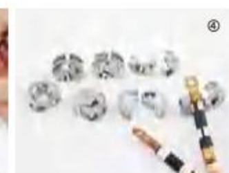
③ 关闭气源，避免误触动而发生危险。用所附送 L 型扳手拆下夹具固定螺钉。 Cut off gas supply. Dismount the fix bolts on the clamp with the L spanner.
