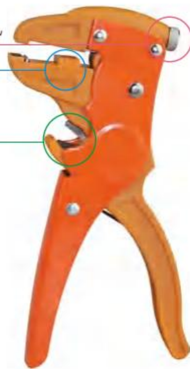
压力调整钮 Pressure adjustable screw
